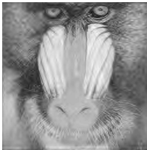
Fig. 4. The compressed image using the mask in Fig. 3. This image requires 4 KB, while the original requires 262 KB
